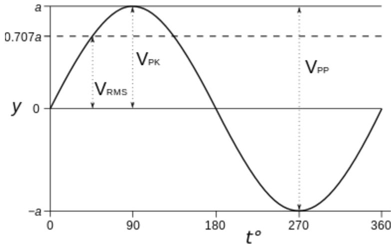
Figure 1 Graph of a sine wave's voltage vs. time (in degrees), showing RMS, peak(PK), and peak-to-peak(PP) voltages
