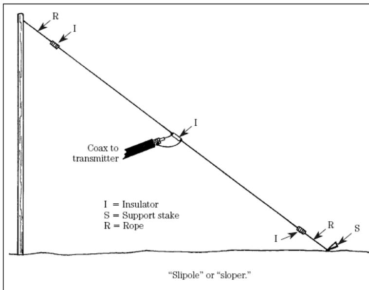
This configuration can be very useful when you have less than the ideal amount of horizontal space for a flat-top antenna, or when you wish to use a single support, such as a tree or mast, for the antenna. (If the antenna is
