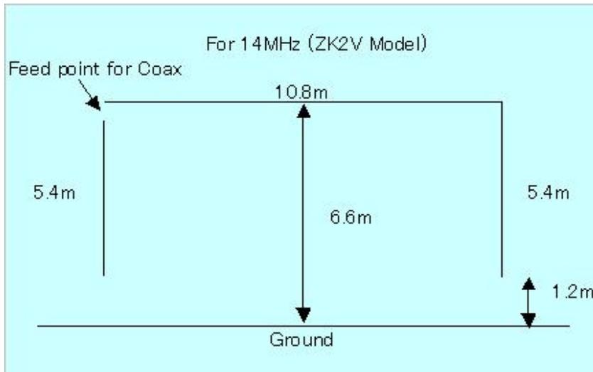
The coax is fed as indicated, with the center wire connecting to the long feedline/vertical, and the shield connecting to the other vertical. You may want to devise a means of strain relief for the coax corner, or some form of insulator. The typical design calls for  $\frac{1}{4}\lambda$  (wavelength) for the two vertical
