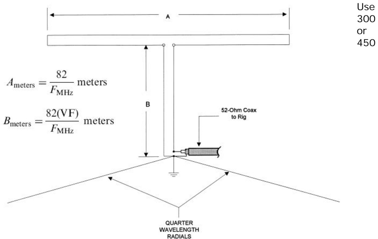
Ohm twin-lead wire, cut to the approximate length needed for the band you want to use (remembering to leave it a bit long to trim down as needed!). There are two main sections of wire, A and B, both relatively the same length. The difference between them is that B is shortened a bit based on the velocity factor of the twin-lead being used. A suggested starting point is a velocity factor of .82 for 300 Ohm wire.
