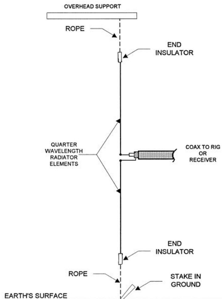
As an aside, in terms of comparison to more common vertical designs, computer modeling shows about a 1.5 dB gain for a HVD over a typical quarter-wave dipole because it is stronger out to the horizon. If you can erect a true half-wave dipole it is definitely worth it!
