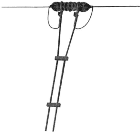
The antenna length can be anywhere from  $\frac{1}{4}$  wavelength to  $\frac{1}{2}$  wavelength and operate successfully, but shoot for  $\frac{1}{2}$  wavelength if possible for best results. Because the antenna is designed to work with multiple bands you will want to use a tuner. Some tuners accept open-wire directly, while others will require a balun to transform it to a coaxial line input.
