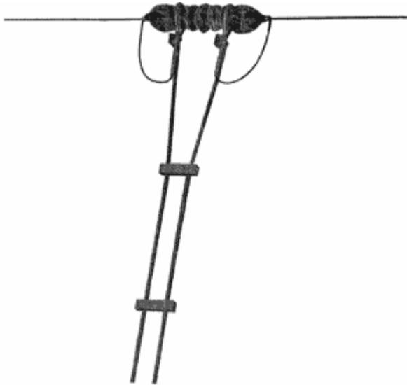
The antenna length can be anywhere from  $\frac{1}{4}$  wavelength to  $\frac{1}{2}$  wavelength and operate successfully, but shoot for  $\frac{1}{2}$  wavelength if possible for best results.
