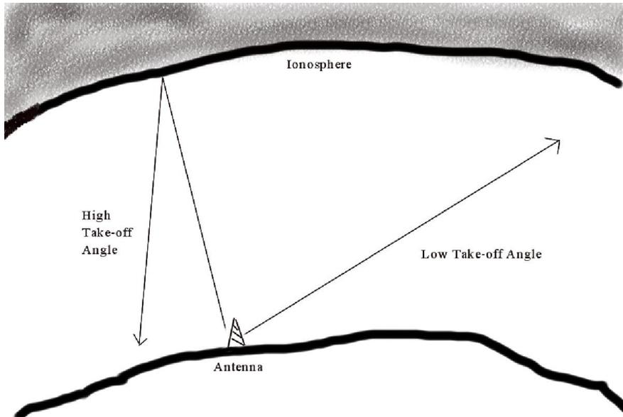
While some RF energy is absorbed into the ground regardless of the take-off angle, DX operators shoot for low take-off angles which allow for the greatest travel distance for their signals.
