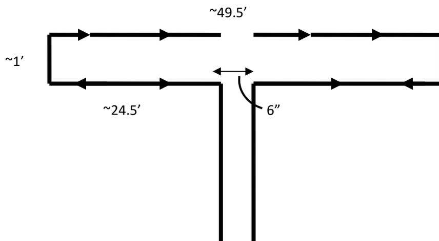
The main advantage of these antennas besides the feedpoint impedance is that they will have a wider bandwidth than their single-wire cousins, with the three-quarter-wave antenna being slightly more directional.
