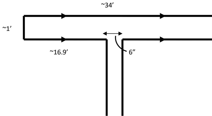
A variant of this which more closely matches the 450- $\Omega$  ladder line is the three-quarter wave 2-wire antenna:
