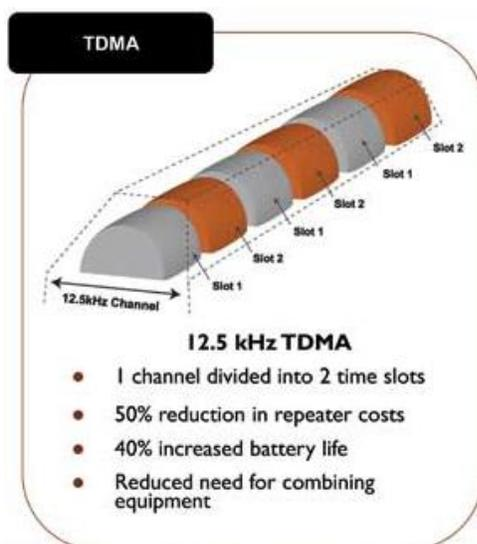
One of the principle benefits of DMR is it enables a single 12.5kHz channel to support two simultaneous and independent calls, achieved using TDMA. Under the DMR standard, Time Division Multiple Access (TDMA) retains the 12.5kHz channel width and divides it into two alternating timeslots A and B where each timeslot acts as a separate communication path.
