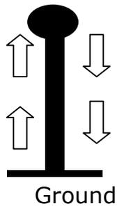
Near-Field Reactance can boost signal strength or weaken it depending on whether or not the reflected signal is in phase with the radiating current.
