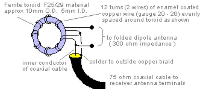
Note - the whole assembly can be mounted in a plastic 35mm film canister. Fill with silicone sealant to waterproof the balun.
