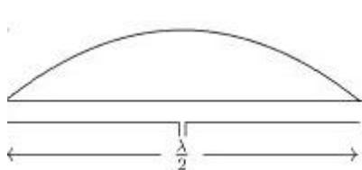
is two wires of equal length connected by a feedline. These antennas are usually measured in terms of  $1/2 \lambda$  – that is, the total length of the antenna is equal to one-half of a given frequency's wavelength.
