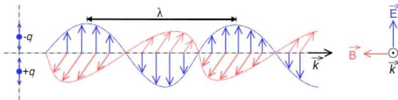
**The blue lines represent the electrical field (vertical plane) while the red lines represent the magnetic field (horizontal plane).**
