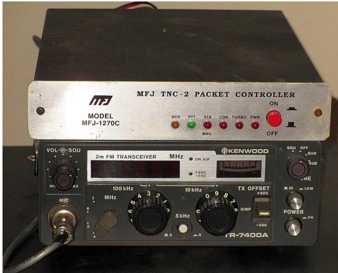
Setup can be a bit tricky depending on whether a radio has its own terminal node controller (TNC) or an external one is used, or if the sound is ported to a computer where software emulates the TNC. My initial APRS setup was with an old MFJ-1270C and a Kenwood TR-7400A (yes, with *dials* and *switches* for each part of the frequency tuning) which I bought as a set from a fellow who was cleaning out his shack. I will not get into all that I had to do to
