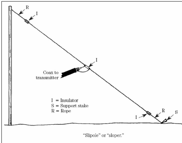
This configuration can be very useful when you have less than the ideal amount of horizontal space for a flat-top antenna, or when you want to use a single support, such as a tree or mast, for the antenna.
