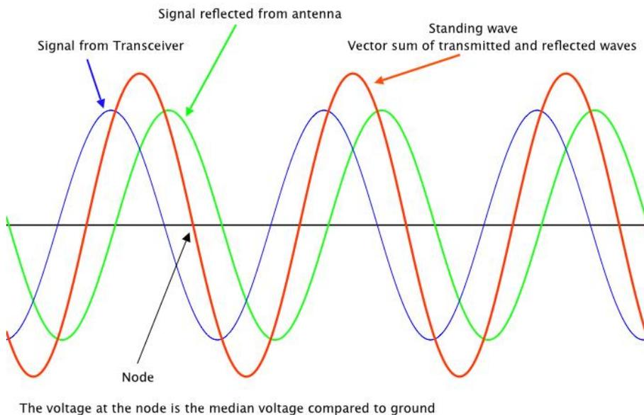
Losses by SWR mismatches don't actually account for much overall line loss, but when coupled with inadequate coax (that is, coax with insufficient matched-line loss ratings), the losses can get quite high. -- And this assumes coax which is in perfect shape—no tears, shorts, or line RF pick-up along the way.
