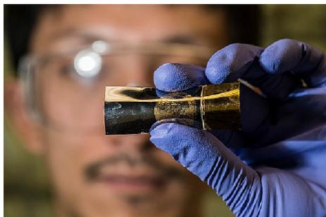
around a solid electrolyte, creating a high-energy battery/supercapacitor. The battery does not need to rely on lithium, and is extremely thin, coming in at about one-hundredth of an inch. Capacity can be increased by enlarging the material or by adding more layers.
