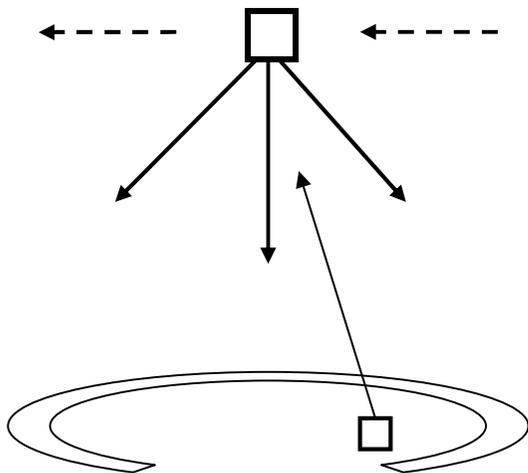
Think of the satellite as an antenna mounted way up high and you will get the idea. Just as an antenna mounted on a high mountain reaches far greater distances than one at sea level, so too an antenna in space reaches far more areas with less power than an earth-bound antenna.
