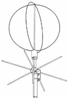
These antennas are designed to deal with the problem of fading by having two loops at a 90° angle to one another. This somewhat replicates an antenna with both vertical and horizontal polarization, so fading is reduced. This is a good solution particularly if you desire to have a station with fixed antennas.
