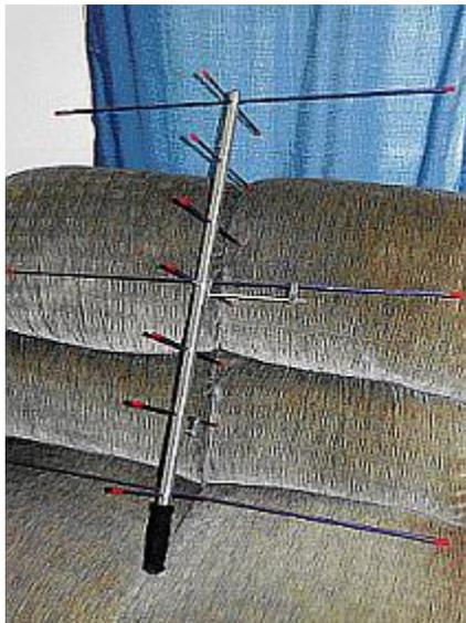
I use a dual-band Arrow antenna, a commercial unit and one that has garnered a great reputation for working satellites (see photo at left). While I would not hesitate to build my own these days, I got this soon after getting into Amateur Radio because I knew working satellites was one of my major goals in the hobby. The antenna does work well, and I have had good customer service from the company.
