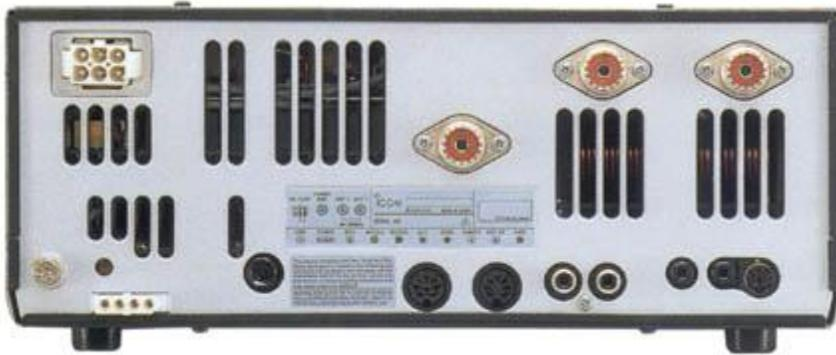
The back of a typical base radio has connections for CAT control (computer command control of the radio), one or two data ports for things like digital modes, amplifiers, etc., and other connections
