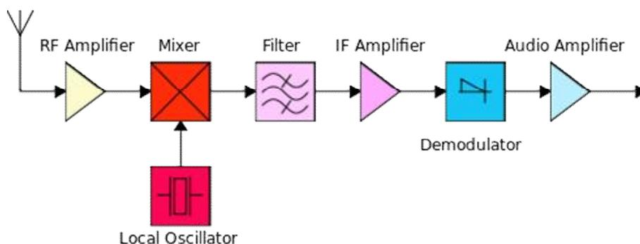
combined, to produce a third frequency. This third frequency is allowed to pass through the radio out to the speaker, while the other elements are not.
