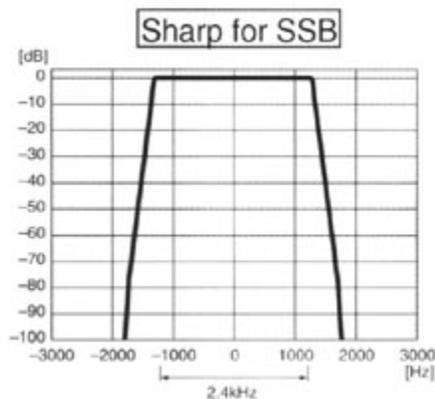
The advantage to passband tuning is that instead of simply narrowing the passband, and thereby reducing the clarity, a usable filter width can be maintained while cleaning up a signal or moving it away from interference.
