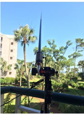
whips, etc. It truly is a marvel of engineering. I used a coil at the bottom of the vertical, followed by a dipole arm, and a telescopic whip. There is even a wire assembly for creating a counterpoise that you can tune simply by varying the length. This proved to be the ticket for this operation.
