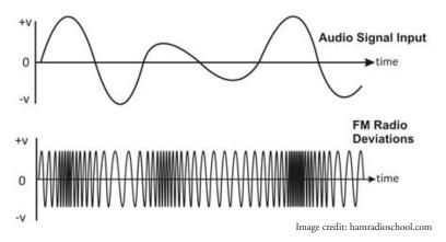
Note that the amplitude of the waves remains constant, only the frequency varies. The loudest audio (see the two peaks near the beginning and end of the graph) result in the highest frequency (dark areas in the FM graph where the waves are packed closely together). The lowest audio input results in the lowest frequency, with the waves farthest apart on the graph.
