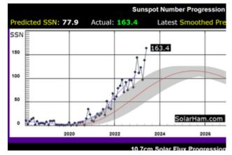
Solar intensity, which is the major factor affecting HF signal propagation, varies in a cycle of approximately 11 years. The previous minimum occurred in 2019-2020, and NOAA predicts the next maximum to happen in 2025, as shown on the above chart. The red line is the government prediction of sunspot activity issued at the beginning of the Cycle, with the grey band representing what was considered to be the likely margin of uncertainty.
