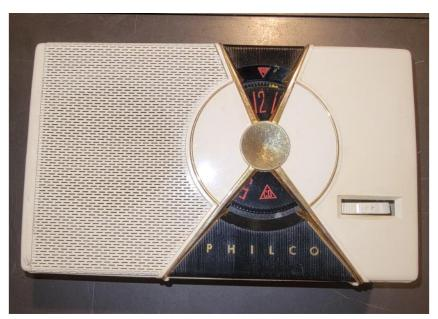
◆ A fully operational Philco transistor radio (batteries included). Based on photo comparisons, this appears to be a T-7 Code 126 or something very similar in appearance.
