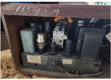
♦ A project piece: Motorola Model 6T Type No. 6-2 combination broadcast AM/shortwave receiver. This item will likely require some work to make it operational. The cabinet has some stains on it and a knob is missing. If you are looking for a piece of radio history and/or a restoration project, this radio could be for you.
